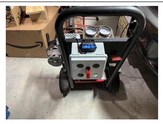
I also included a tachometer and time run meter. It senses the spark via a wire wrapped around the spark plug cable. The red toggle switch in the center allows the engine to be started with no load. As soon as the engine starts, you flip the red switch up to start the alternator output. The large DC switch on the right disconnects power to the instruments and outputs. All wiring is fully fused along with 100 amp links in the main power cables.
