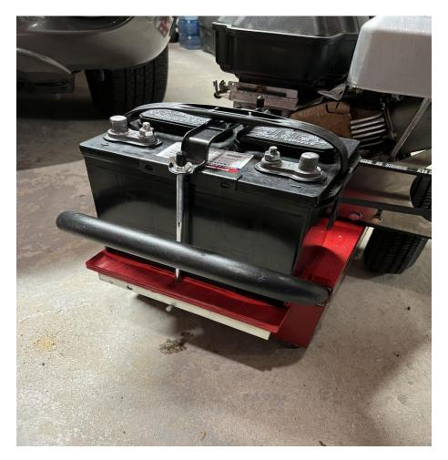
I found that if the engine is turning at approximately 2000 RPM the alternator is turning at 2700 RPM. According to the vendor test records, 2700 RPM is good for about 65 amps output. So far the unit has been load tested to 60 amps with no stalling.
