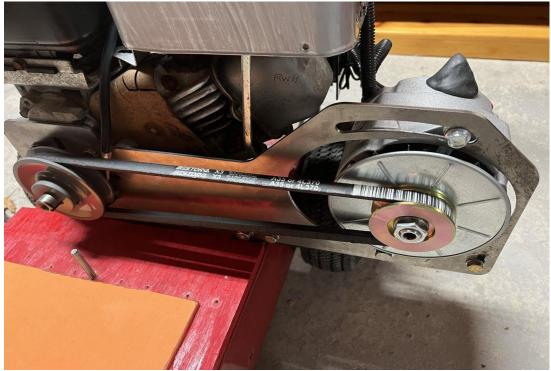
It is important to fabricate and install a belt guard to prevent anyone or anything from being caught in the drive system. See the guard below
